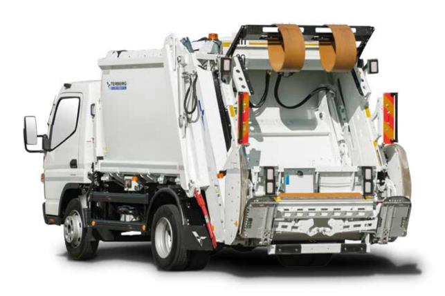
Olympus Mini is a rear loading refuse compaction vehicle for the collection of domestic and organic waste as well as recycling materials in pedestrian, city centre and rural areas with narrow streets and restricted access that requires a high level of manoeuvrability. Compact, with an elegant design and proven technology, offers the best quality and reliability for the most demanding waste collection experts.
